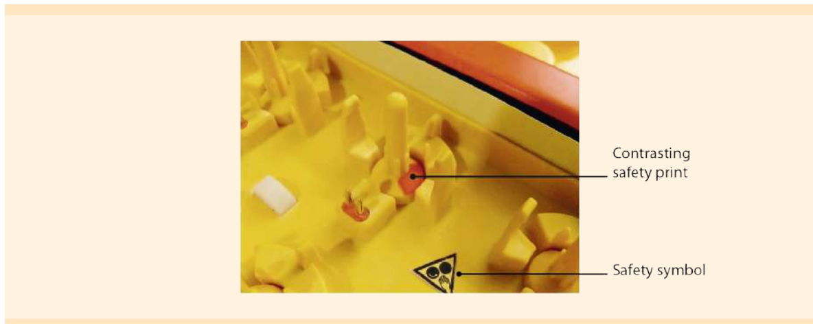
Figure 1: Safety symbol on the Trough of the gentleMACS Octo Dissociator with Heaters. The Sleeves are marked with a contrasting safety print.
