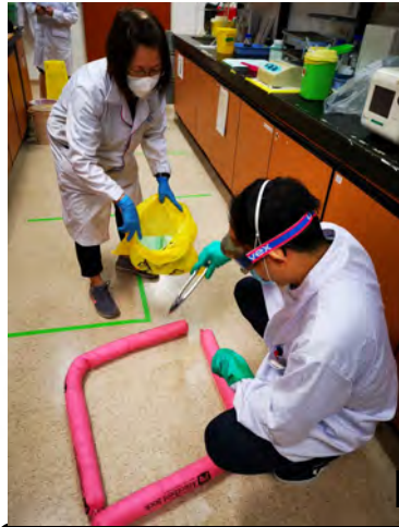
STEP 7: A. Place all contaminated materials into chemical waste bag
