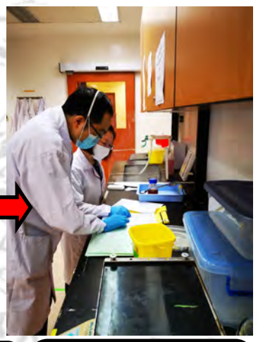
STEP 3: A. Check Safety Data Sheet (SDS) B. Demarcate spill area to minimize cross-contamination
