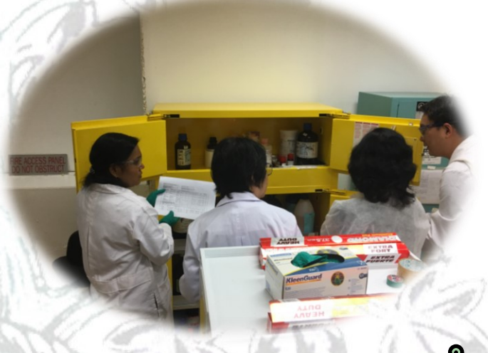
Checking of flammable storage cabinet to ensure the MAQ is not exceeded
