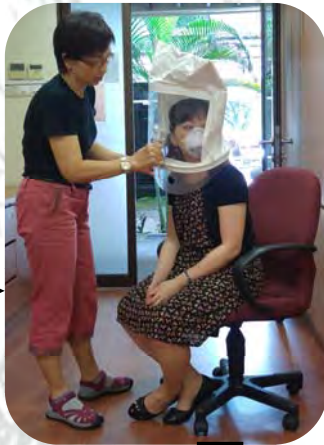
2. Put the space suit and spray inside to check suitability of the mask
