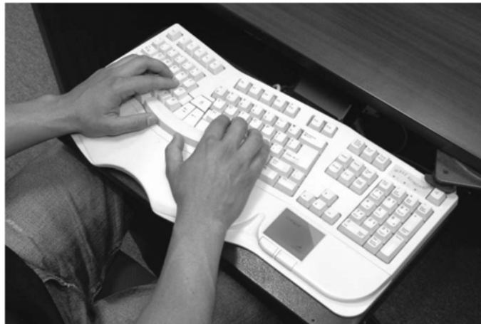
Figure 17: An example of a split keyboard which allows for neutral wrist and arm posture.
