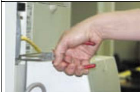
Use of a tool handle when the hand force is applied horizontally
