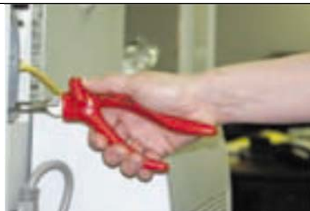
Use a tool with bent handles when the force is applied horizontally (i.e., in the same direction as your straight forearm and wrist).
