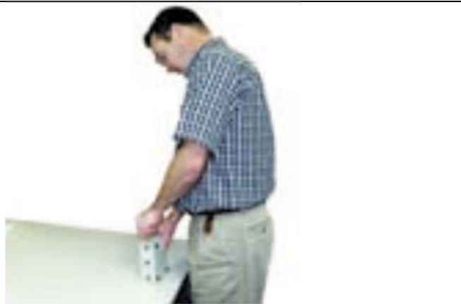
Reposition the workpiece (above) in such a way that the arm and elbow will be at the same level of the work surface. Working also on a lower work surface (below) will help avoid bending of elbow and arm.
