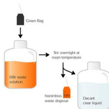
Figure 10.3 Absorption System for Ethidium Bromide Decontamination
