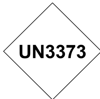
Diamond-shaped mark for “Biological Substance, Category B” and for genetically modified microorganisms and organisms that meet the definition of an infectious substance, Category B
