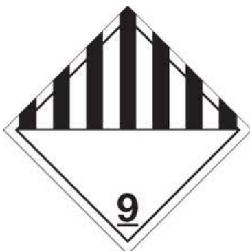
Hazard label (Class 9 Miscellaneous Dangerous Goods) for certain noninfectious genetically modified microorganisms and organisms (UN 3245) and for dry ice (UN 1845)
