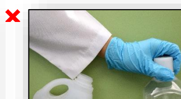
Fig 2: Loose lab coat sleeve knocking chemical container
