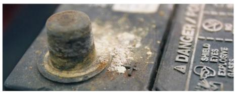
Figure 11: Lead sulphate deposits on battery connector
