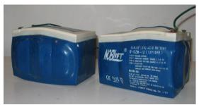
Figure 12: Bloated lead acid batteries
